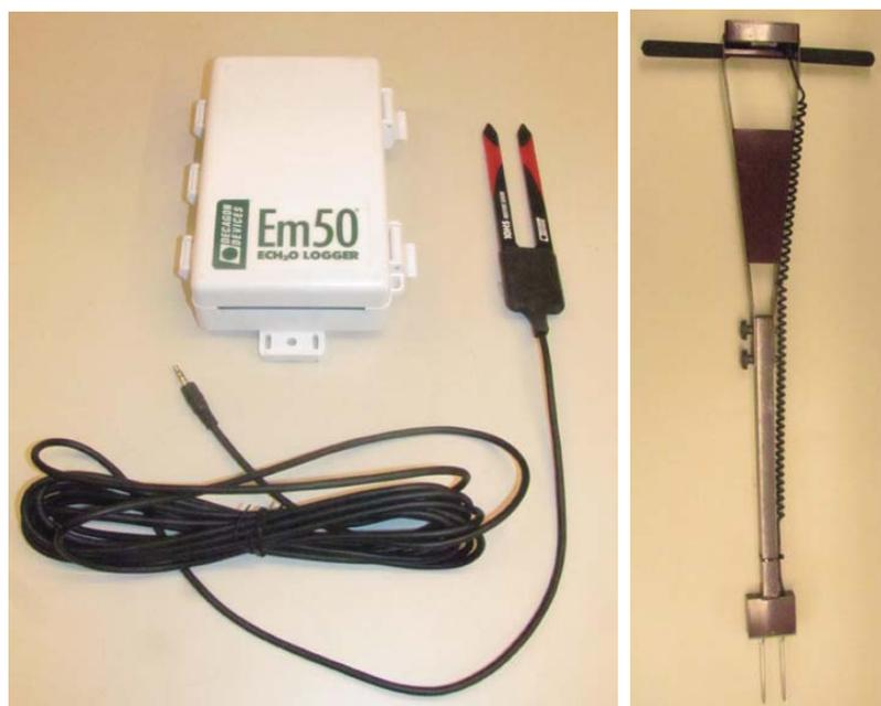
**Figura 4.** a. Sensor FDR y registrador (Decagon). b. TDR 300 (Spectrum Technologies).
